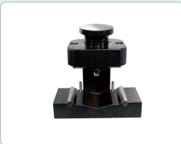
cementitious sand flexural fixture (included)
